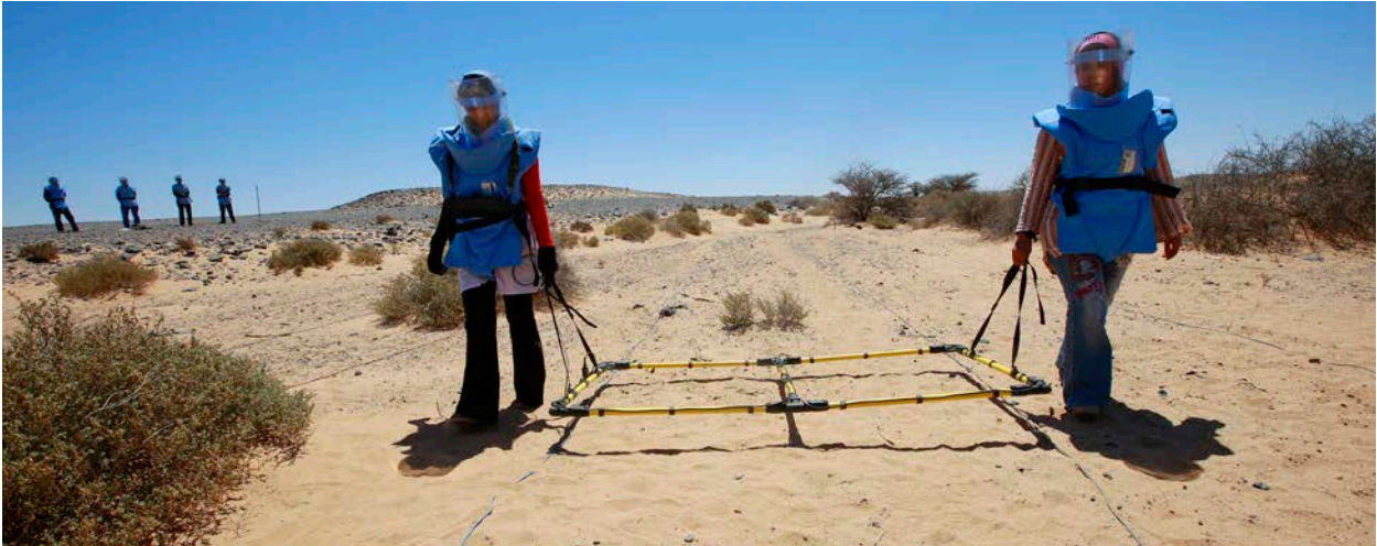
Women Battle Area Clearance (BAC) operators from non-governmental organization Action on Armed Violence, working under a contract from the United Nations Office for Project Services (UNOPS), use a large loop detector to locate mines in Mehaires, Western Sahara. 17 June 2010. UN Photo #440156 by Martine Perret.
